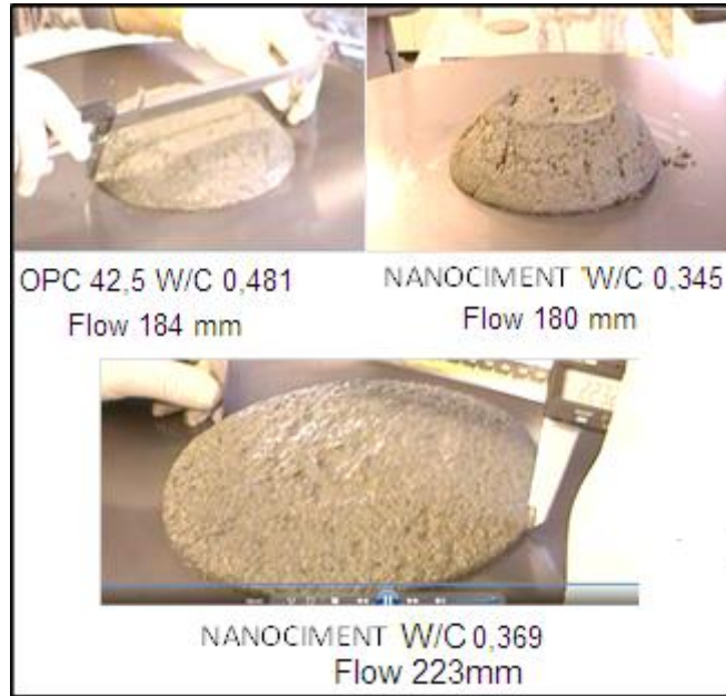
Figure 3.3 – Consistency of Nano-cement and (OPC 42,5) cement measured at flow table
